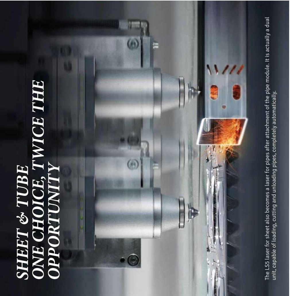
The LS5 laser for sheet also becomes a laser for pipes after attachment of the pipe module. It is actually a dual unit, capable of loading, cutting and unloading pipes, completely automatically.
